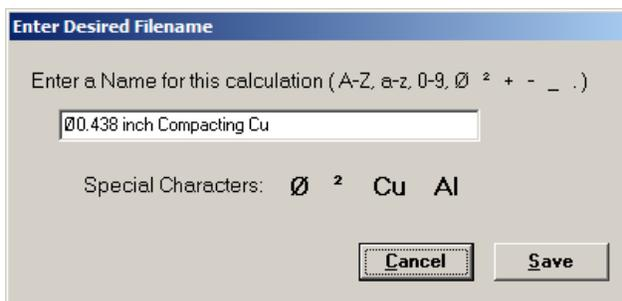
The **Save As** template has been designed to assist in quickly creating a suitable filename for a CR calculator. For example, if a Ø0.438 inch compacting die is featured in a calculation, the filename may be entered as shown. Or it may be desired to give a name such as “240 mm<sup>2</sup> Cu Cable”. The special symbols Ø and <sup>2</sup> may be inserted into a filename just by clicking the corresponding
